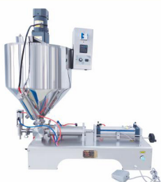
Single head paste filling machine with heater and mixer
