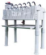
12 Heads corrosive liquid filling machine
