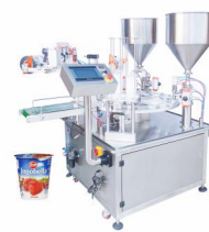
Yogurt and jelly cup filling and sealing machine (two filling station to fill different liquid)
